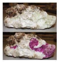
Figure 1: The mineral hackmanite from Greenland – before and after exposure to ultra-violet light
