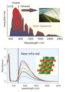
Figure 4: Top: the solar spectrum showing the large component in the IR region; inset a poly-tunnel greenhouse which frequently overheats due to such radiation. Bottom: the near-IR absorbing properties of some new pigments showing practically no absorption in the visible region; inset the structure of new IR absorbing pigment
