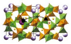
Figure 2: Schematic showing the key structural elements of hackmanite that allow it to change colour – an electron (represented by an orange-brown sphere) is transferred from the ion (magenta) on the cage on the left and becomes temporarily trapped
